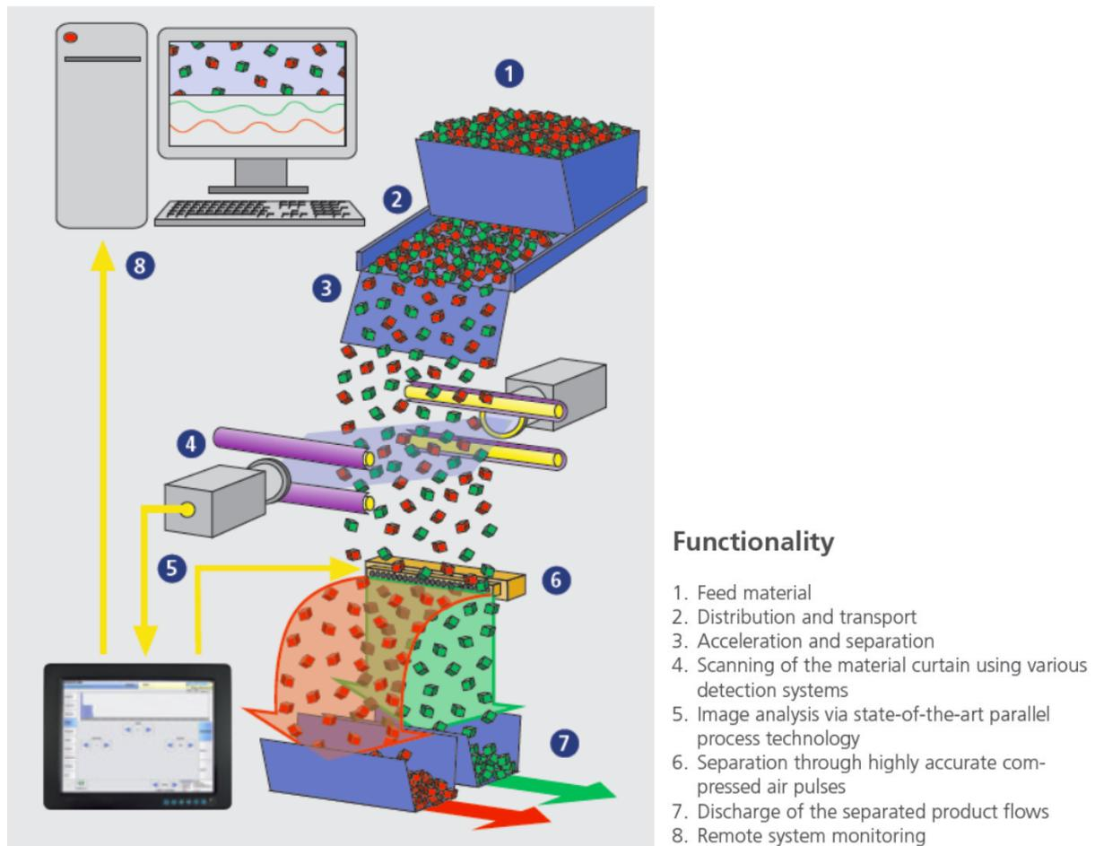
Picture: 2: Ejection with pneumatic / compressed air pulses (source: Allgaier)
