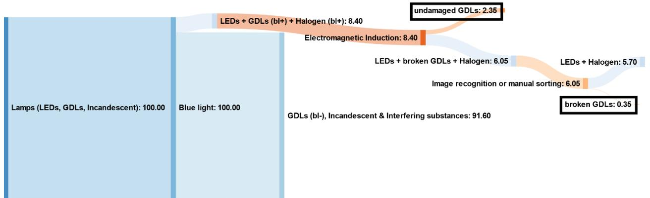
Figure 12: Sankey diagram for testing starting with blue light with electromagnetic induction as second step
