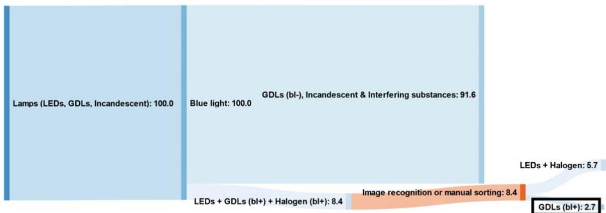
Figure 14: Sankey diagram for testing starting with blue light with only manual sorting as second step
