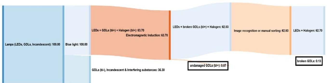
Figure 13: Sankey diagram for future scenario with blue light with electromagnetic induction as second step
