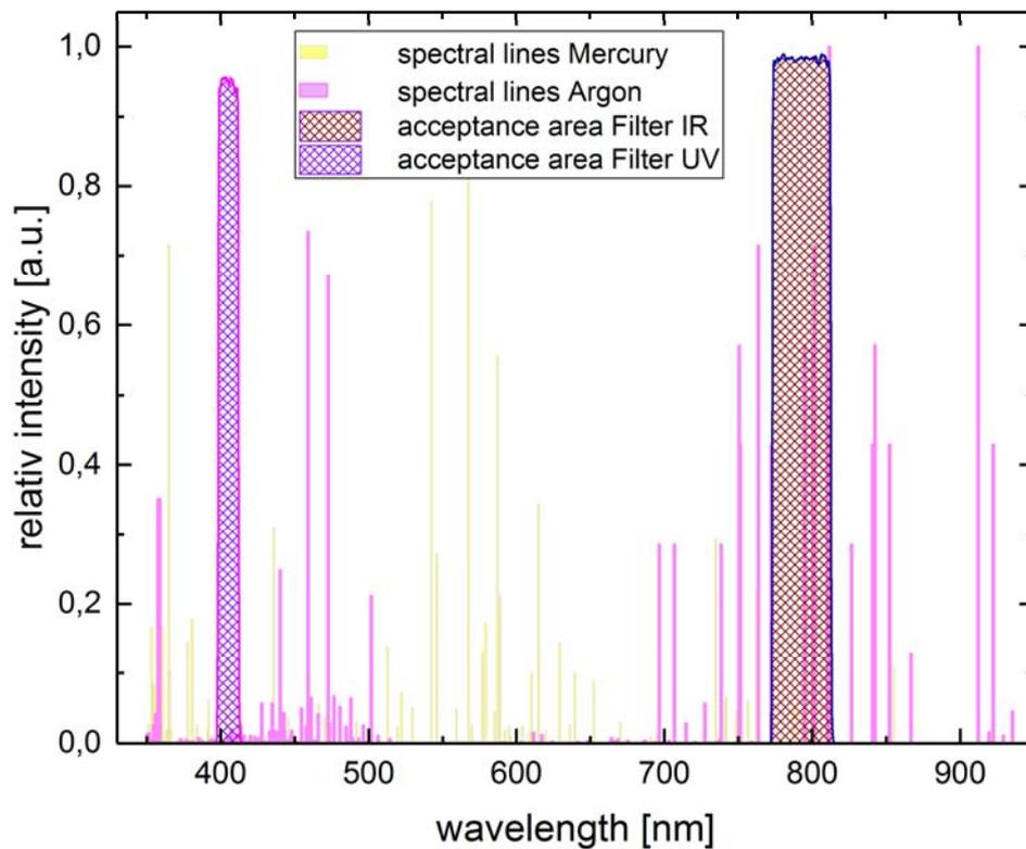
Figure 7: Optical bandpass filters with spectral lines of Ar and Hg
