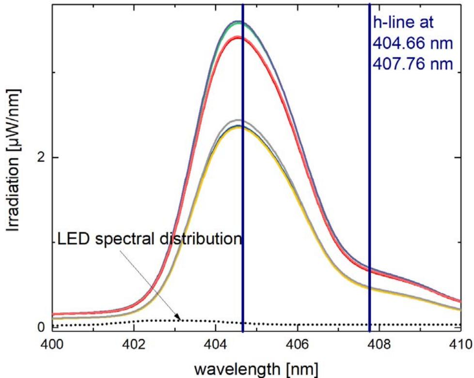
Figure 4: High-resolution spectral measurement on GDL and LED in the h-line region
