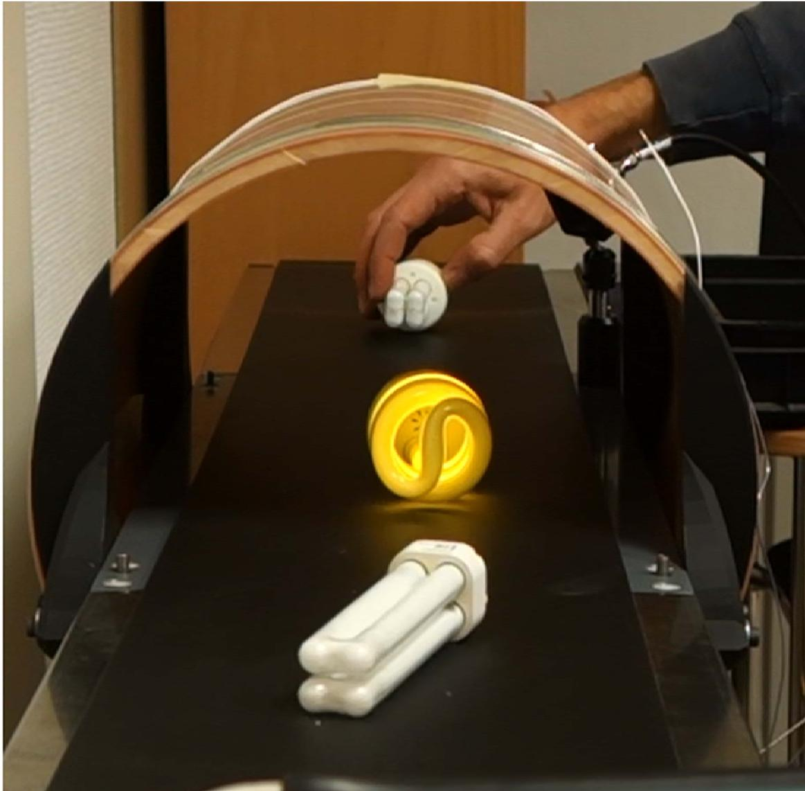
*Figure 19: Prototype of conveyor belt with devices under test, partly showing fluorescence*
