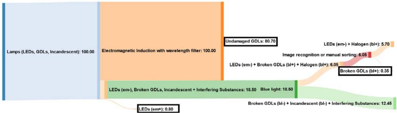
Figure 8: Sankey diagram for testing starting with electromagnetic induction including wavelength filter
