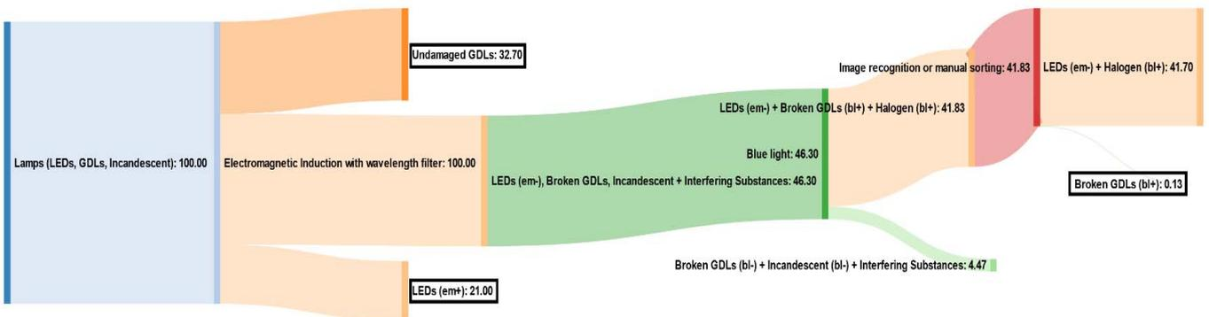
Figure 9: Sankey diagram for future scenario starting with electromagnetic induction including wavelength filter
