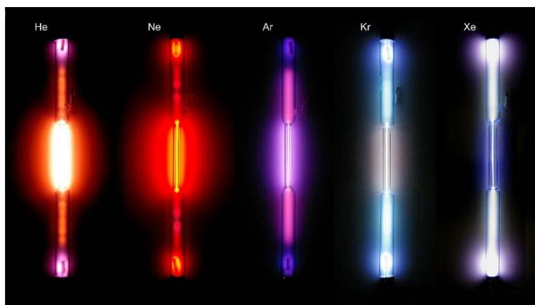
Figure 5: Noble gas-discharge lamps in operation
