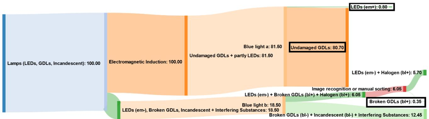
Figure 10: Sankey diagram for testing starting with electromagnetic induction including blue light twice
