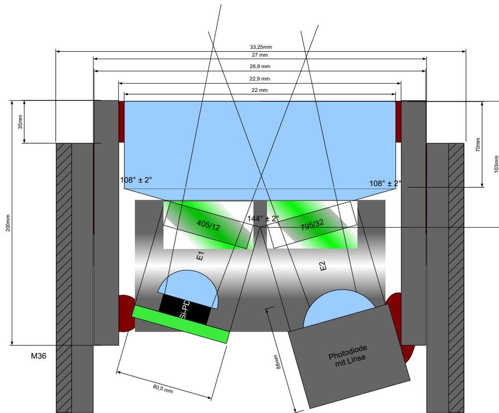
Figure 8: Mechanical concept of an optical sensor head
